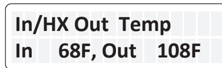
Figure 41. Inlet and Heat Exchanger Outlet Temperature
